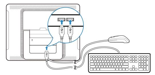
1. Connect the USB cable on the keyboard to a USB port on the rear panel of the computer.
